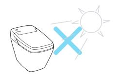
Do not cover the seat sensor, body detection sensor, and remote control transmitter and receiver.
