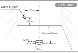
Set out (S-Trap) 150-350mm. Flexi pipe may be required. Standard set out 305mm.
