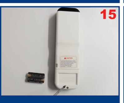
Unscrew battery cover and place in batteries.
